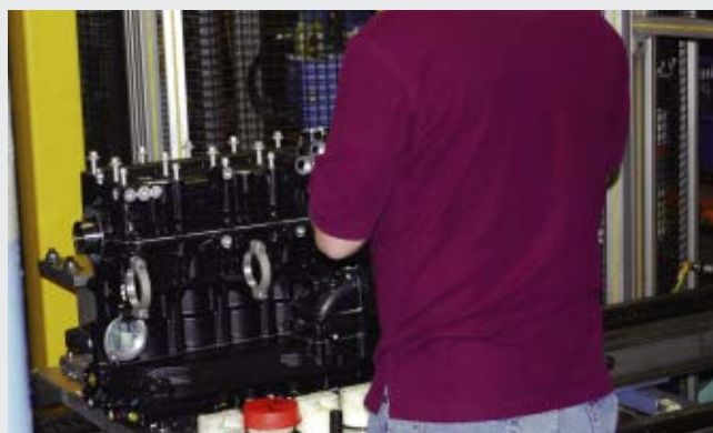
This is an automated station where the crankcase sealant is applied by a robot. It used to take 12 hours to build an engine but now they can build a Verado in 3 hours. Verado models from 135 to 300 and the 350 horse high-performance motors are all built on this one line by selecting different parts. At this point, an operator will add the long bolts (which are up to 14 inches long) and hold all the parts in compression as they add the crankcase to the block on the head.
