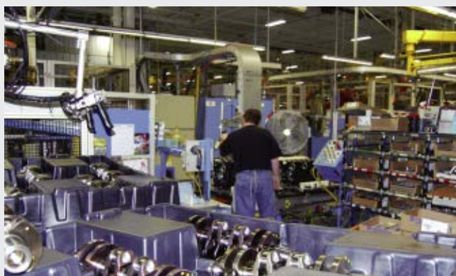
Quality control tests are conducted at all points. Pistons are checked for specifications as they are selected. Since the engine is built from the head up, this technician uses an auto-oiler as he inserts the pistons. At the next station, a machine picks out the crankshaft and bearings. Lights guide the operator on which one to select. Next the rod and cap assembly and minor parts are added.
