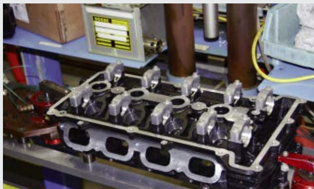
The short block, or green power head starts with the head assembly positioned in a jig. The aluminum and steel machining is done here in Fond du Lac, Wisconsin.
