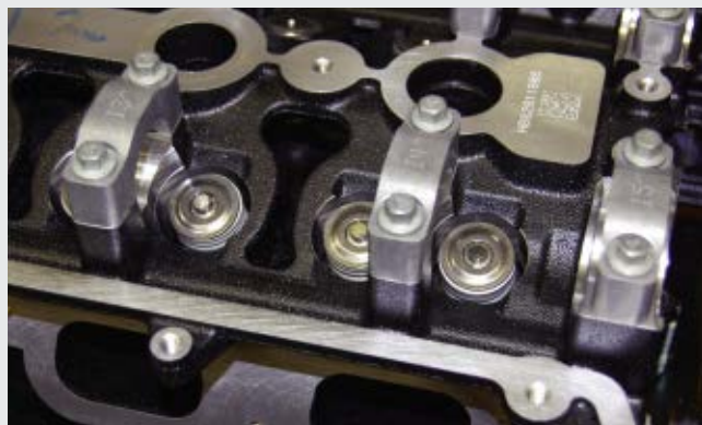
Process control is where the technicians collect the "birth history" of the engine and sensors track the assembly process to ensure completion of tasks like adding the proper lubrication before the part moves on. The system will physically not release a part until it has met all the necessary steps. Here, the valve keepers have been added. Other steps are where lasers scan and leak test the combustion chamber and ensure that valves return correctly.
