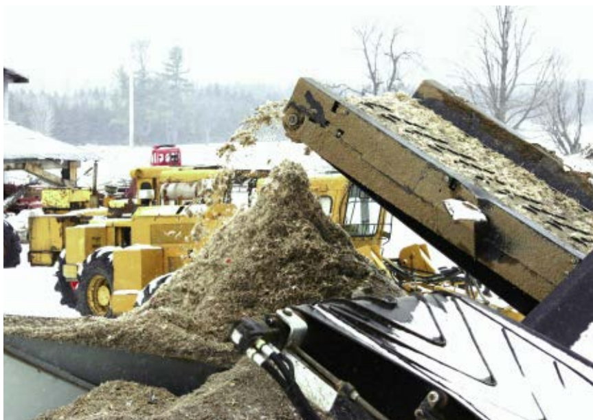
Immediately after the shredder starts its work, the byproduct begins to appear – shredded fiberglass.
