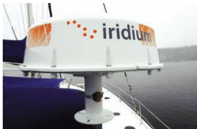
Iridium OpenPort 1: Open Port by Iridium is one solution to getting internet onboard but these were developed for commercial use and may be too large an antenna to suit mid-range recreational boats.
