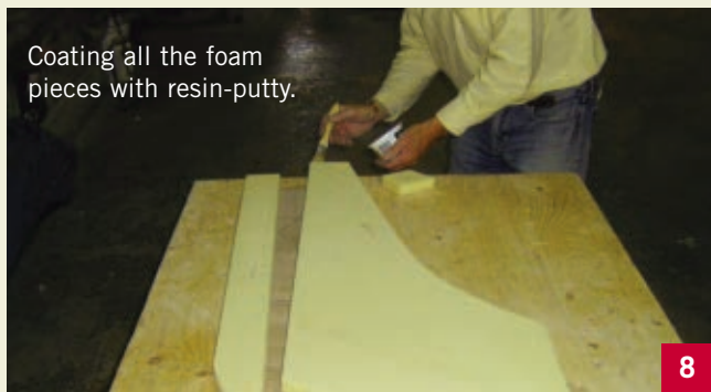
Fastening the foam pieces with resin-putty and screws.
