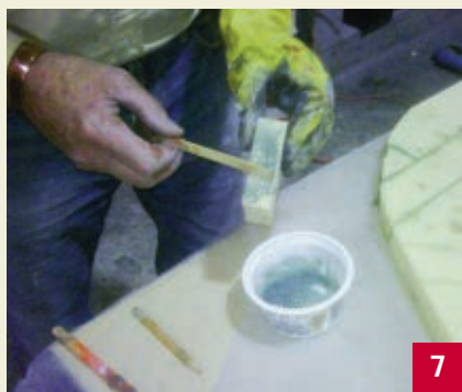
Coating all the foam pieces with resin-putty.
