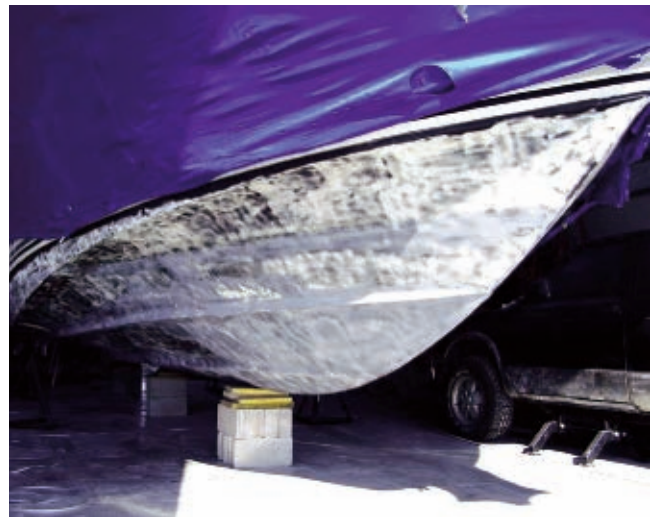
Bottom paint removed.
