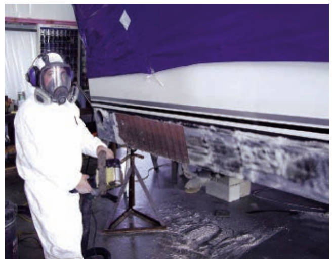
Peeling off old gelcoat.
