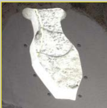
Although we made a template of the engine cutout and bolt holes, the job was made easier by having a Mercruiser template bracket to get an exact fit.
