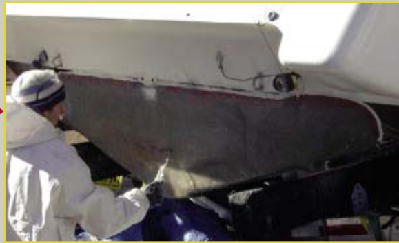
The outer lamination was matched with the original and finished with a layer of chopped strand mat.
