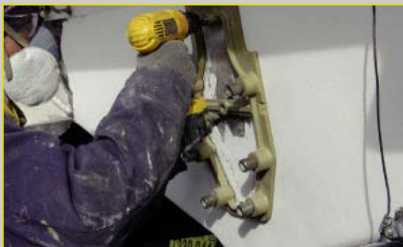
Although we made a template of the engine cutout and bolt holes, the job was made easier by having a Mercruiser template bracket to get an exact fit.
