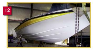
With the repairs and painting completed and the rub strake in place, the boat is ready for final detailing.
