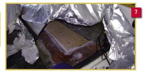
In the helm area the foot throttle pad is bonded in place before being laminating to the cockpit floor.
