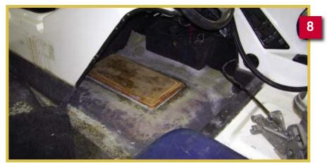
Now that the repaired area has been faired, the first coat of two-part polyurethane white finish is applied and the surface is checked for blemishes and pinholes.
