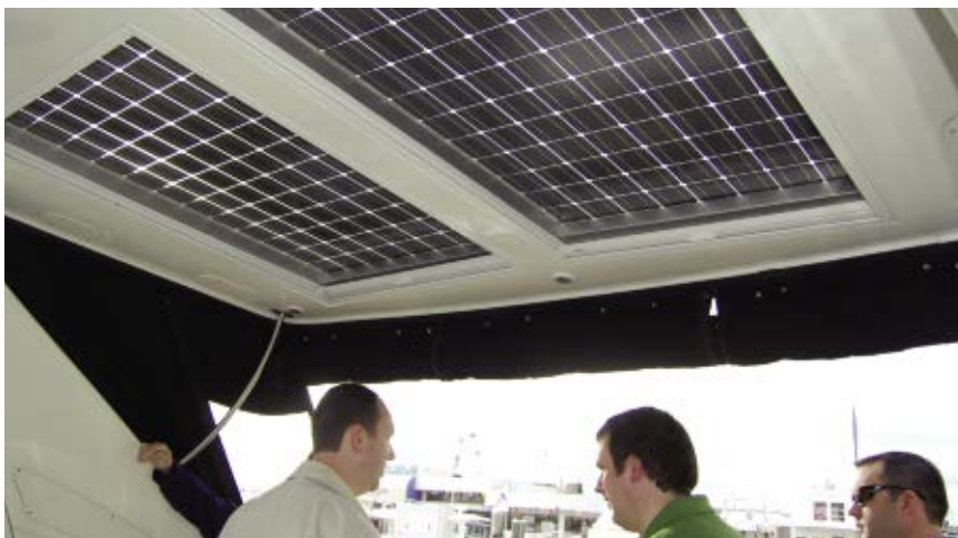
This looks to be a conventional express cruiser hardtop but the two solar panels you see can generate a fair bit of charging power. They work with both direct sunlight and reflected light coming back up off the water.
