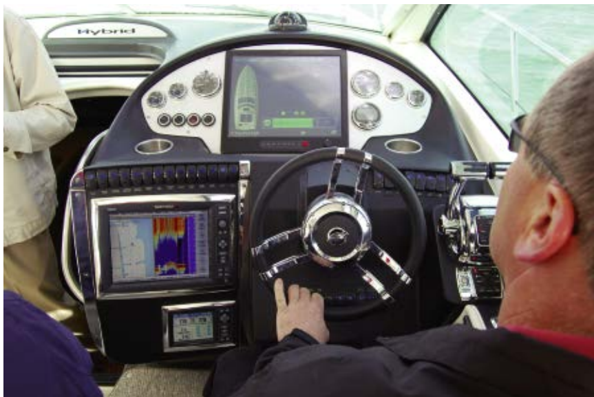
Above: The handsomely appointed helm features Mercury SmartCraft instrumentation and controls, analog instruments for each of the engines as well as the big center-mounted information screen that provides information on all systems.
