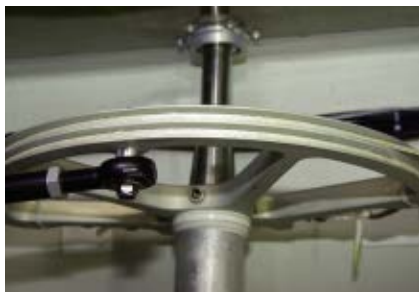
All steering quadrant cables should be adjusted and checked for any excessive wear.
