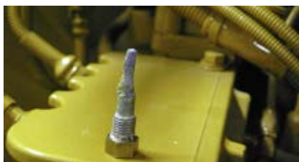
Engine cooling system anodes are often hard to locate and therefore neglected. Failure to replace these in a timely fashion can cause serious damage to engine heat exchangers.
