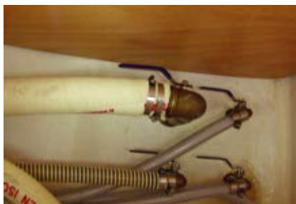
For seacocks with double clamps, it's important to check for free movement and handle orientation to ensure full travel from opened to closed. Regarding double clamps, remember that the ABYC does not require this in H-27. In fact, if the barb on the thru-hull is not long enough to accommodate the full band width of the clamps, double clamping can cause more harm than good.
