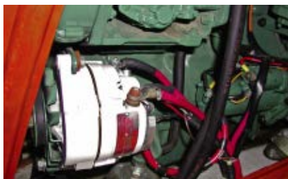
Alternator and starter motor terminals should be protected with insulating boots NOT as shown here. Remember that the starter motor circuit is the only circuit on a boat that is not required to have a fuse installed. If a metal object contacts the terminal and the engine block simultaneously, a serious short circuit will occur, possibly causing an engine room fire.
