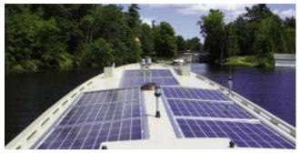
The most visible indication that Sparks is a solar electric hybrid boat comes from the roof mounted solar panels but the handrails on the sides and the sweep of the roof make them barely noticeable.
