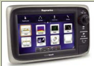
Raymarine's new e7D Multifunction Display features built-in Wi-Fi connectivity and Bluetooth wireless technology including an optional RCU-3 wheel-mounted or handheld remote control unit.
