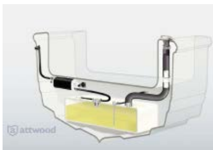
Attwood has supplied this useful diagram showing a correctly installed fuel filler, tank, vent line, carbon canister and P-trap valve.
