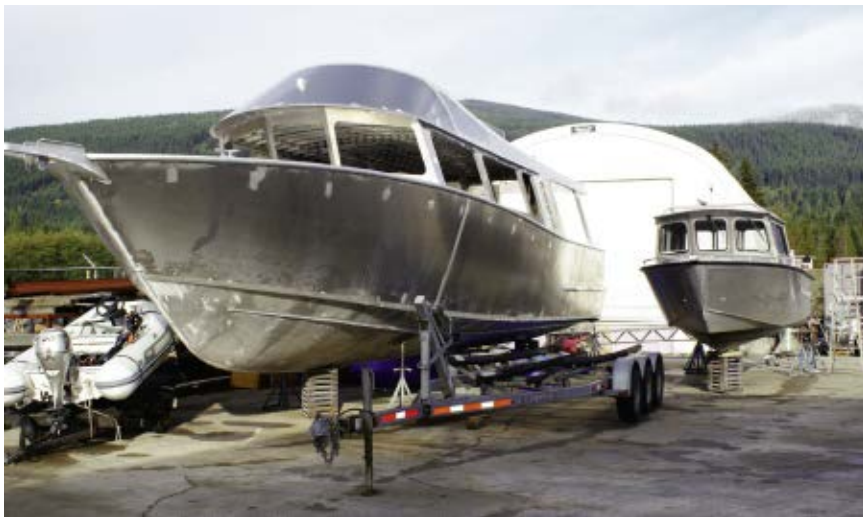
A fully-welded 45' hull and house awaits the paint shop immediately to its stern. The smaller craft to the right is an early model workboat in the yard for repowering.
