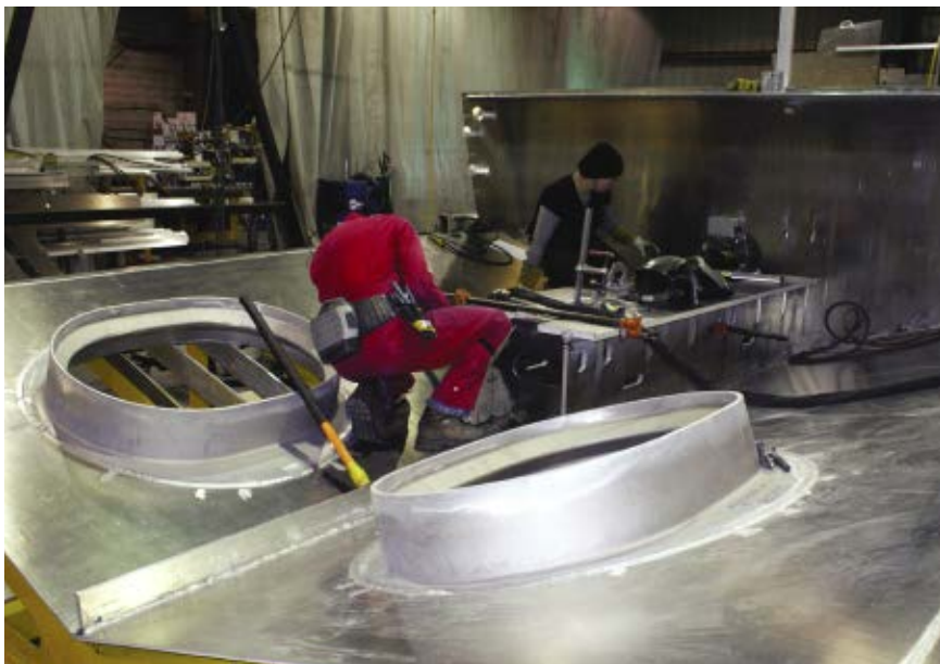
In the engine room of a new 56, the mounts for the IPS drives are newly welded in place and the central bench of the engine room receives final installation welds.
