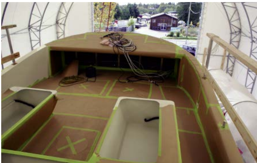
The flying bridge on a 56-footer under construction shows the layout for components to be added later. It's pre-wired with the NMEA 2000 "backbone" (in black) for navigation electronics which are installed last.
