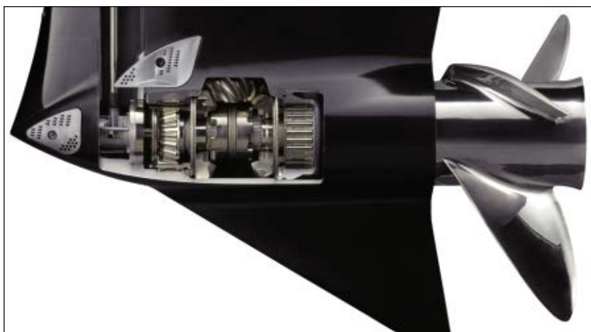
This cutaway shows the clever Suzuki gear set design that allows the dealer to determine the rotation or to change it.
