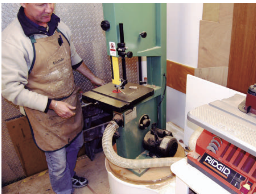
This is really clever; the band saw is on a turntable so it can be angled out for long work or left in for small work. Notice the dust collection hose; a big dust collector is working at all times to keep the environment clean and healthy.
