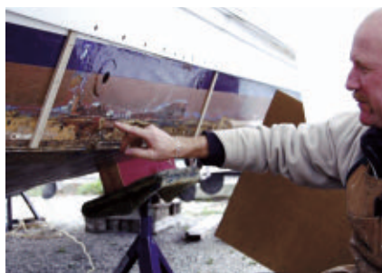
Merv Webb shows me the repair to be done on the Chris-Craft. Wood at the chine was damaged in an accident. When those boards were removed, an area of rot below the waterline was discovered. This type of repair needs to be done by a person with the right skills.
